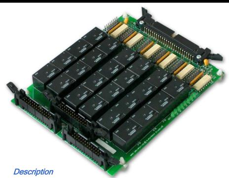
These cards are general purpose 24 channel relay cards. All cards have a 50 way header connector (compatible with NIDAQ DIO24/6503 DIO card) which connects to optoisolated input relay drive signals. All relay contacts are connected to three 26 way header connectors.
